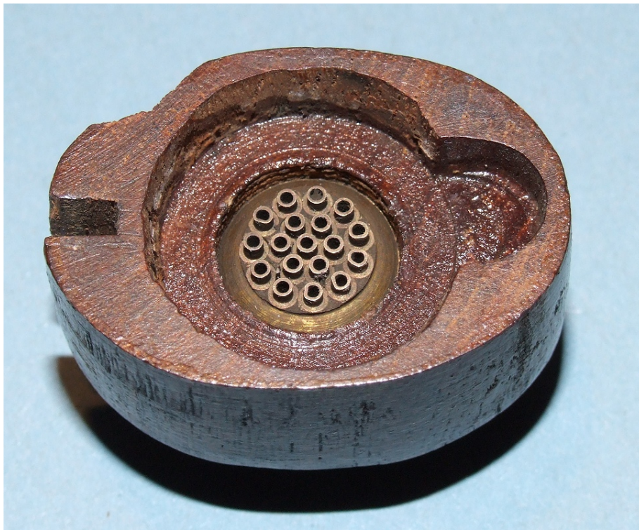
Figure 6b. A "pepper pot" exhaust valve seat (Battersea Town Hall organ) (Copyright © Lucien Nunes)
