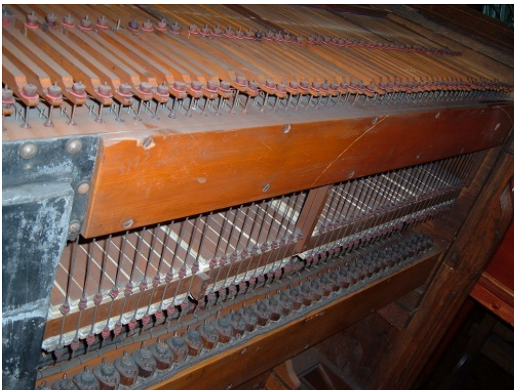
Figure 25. Electropneumatic combination action at St Modwen's, Burton upon Trent
