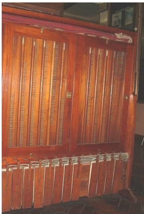
Figure 12. A Hope-Jones coupler relay cabinet (Copyright © Lancastrian Theatre Organ Trust)
