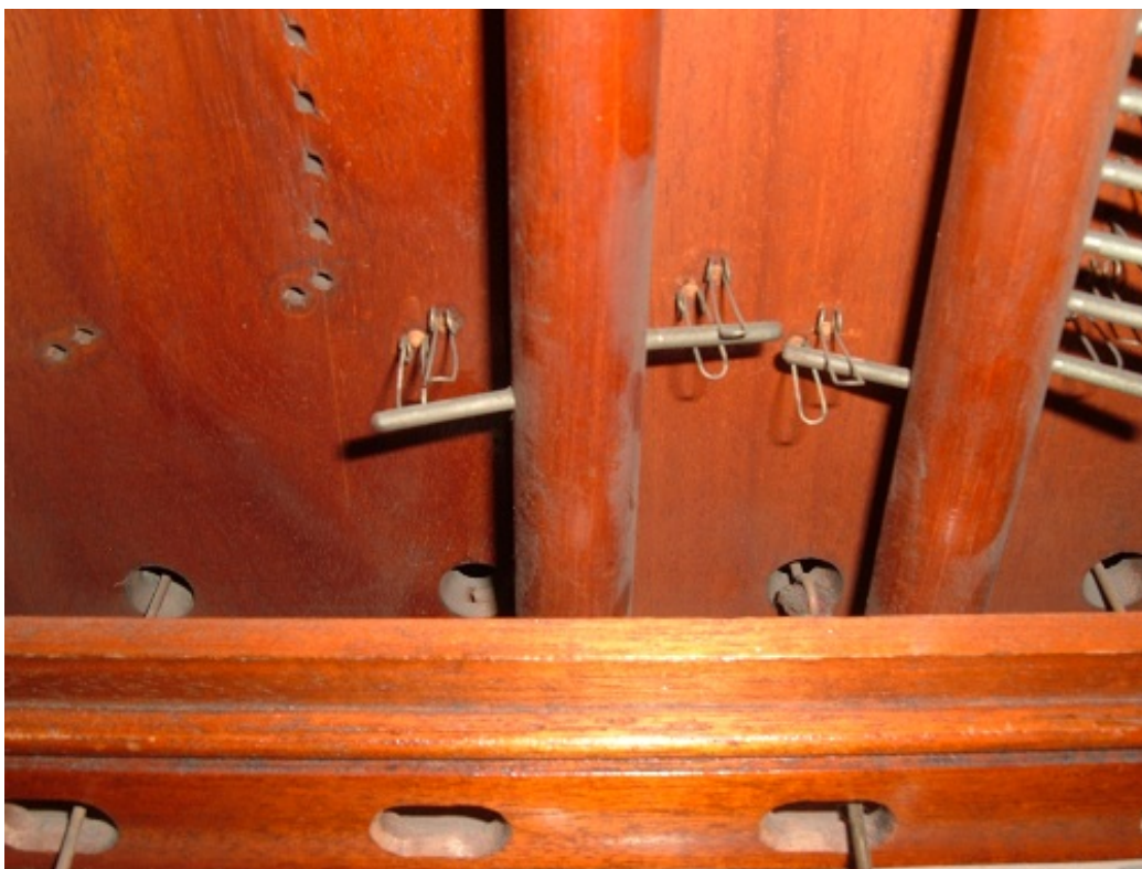
Figure 5. A Hope-Jones coupler relay using wire loop contacts
