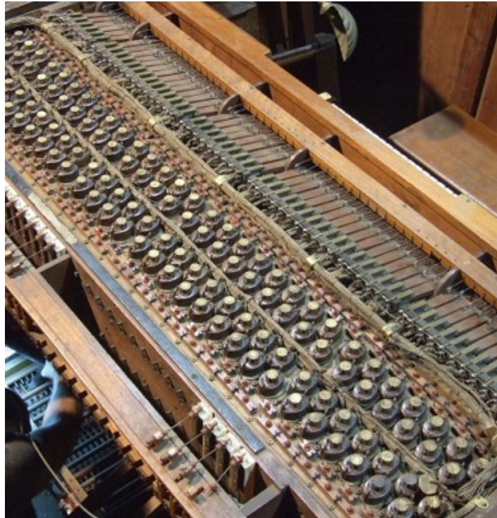
Figure 24. Electropneumatic combination action at Battersea Town Hall (Copyright © Lucien Nunes)
